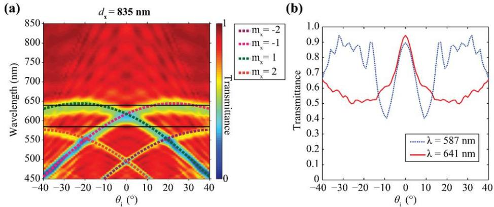
Figure 3. (a) Zero-order angular transmittance map for  $\lambda$ , when  $d_x = 835$  nm. (b) Cross-sectional profiles at the wavelengths  $\lambda = 587$  nm a  $\lambda = 641$  nm. Dashed lines indicate the analytical dependences, Eq. (1).
