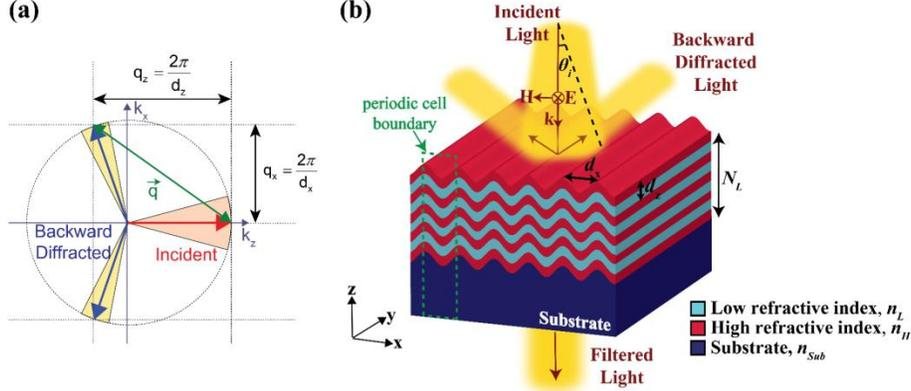
Fig.1. (a) Illustration of the PhC angular filtering in Bragg configurations. (b) Three-dimensional representation of designed PhC spatial filter geometry.
